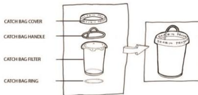
The Catch bags are designed for long life with sturdy materials. If somehow the Catch bag filter has a problem it is easily replaced.
